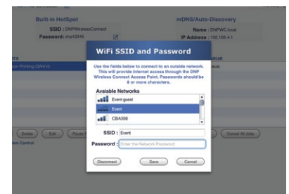
Connect to outside WiFi network to provide internet access.
